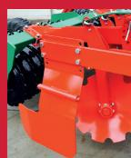
V-Profile double disc roller. Optimum consolidation in stripes as well as in depth.
