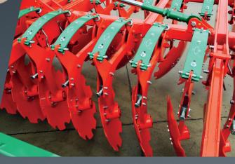
The discs of the *Eurodisc* are set in a very aggressive angle. That is why the quality of the work delivered by the *Eurodisc* is so extraordinary, even with the most
