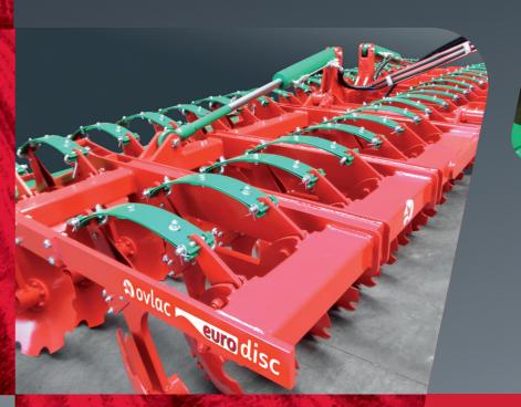
100% maintenance-free sealed hubs. Ovlac 's own design, the disc hubs feature a double conical bearing. This allows that the large 24" discs are held by their inner side which offers a more gentle transmission of side forces towards the bracket on the frame as well as a better protection of hubs from soil projections coming from neighboring discs or wearing from contact with the soil surface.
